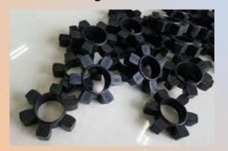
Spider coupling are torsional flexible shaft couplings, the operating characteristics of which are two hubs with concave claws, transmitting the torque by meshing with an elastic involute gear ring.
